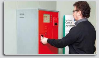
Ticket reading determines the automatic application of the rate. When payment is completed, the machine will return the change (if owed), the receipt (if requested) and gives the user a grace time to exit.
